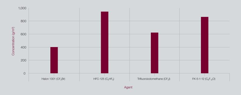
and environmental costs. Implementation of these larger, heavier replacement bottles may require the relocation of extinguishers or adjoining emergency equipment, redesign of interior panel structure, and recertification of extinguisher installations for in-production airplanes and retrofit applications. The increased size and weight of the bottles may also hinder firefighting performance in an airplane cabin.
