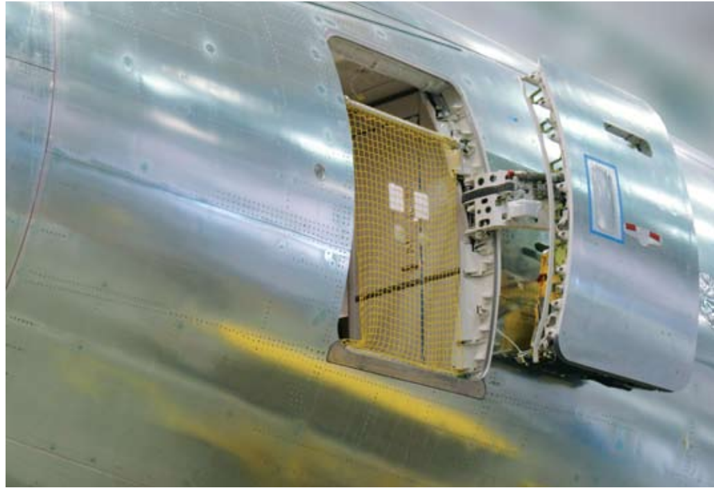
Door safety nets such as these are used on the 777 during production.
